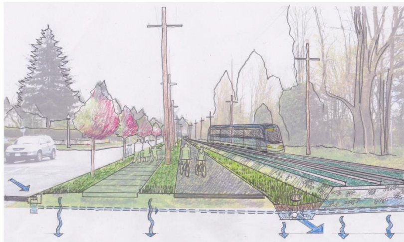
SK-B illustrates sidewalk, separated bike route, infiltration rain garden, LRT with 'green tracks', structural base / STW trench.
