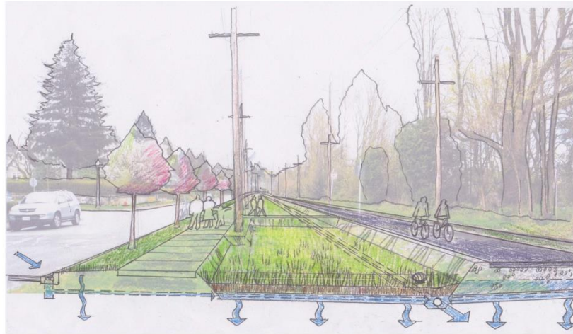
SK-A illustrates sidewalk, rain gardens and interim bike route over infiltration trench with under-drain (base for future LRT).
