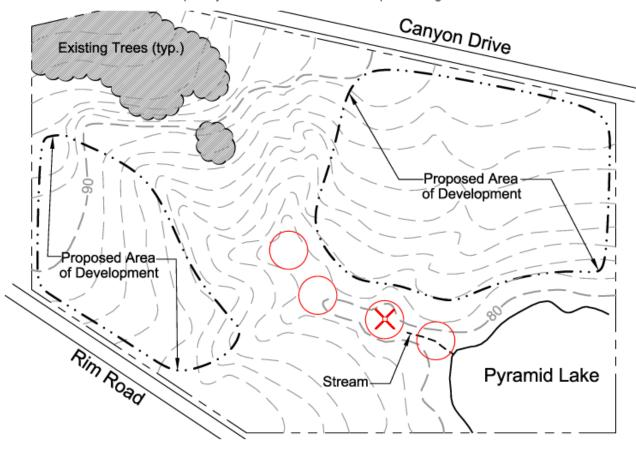
In what order should these construction activities occur from project initiation to substantial completion? Place the activities in order. **CLEAR AND GRUB SITE INSTALL SEDIMENT AND EROSION CONTROLS** PERFORM MASS 3 **EARTHWORK** INSTALL SUBSURFACE 4 UTILITIES CONSTRUCT BUILDINGS AND SURFACE TREATMENTS 6 **ESTABLISH TURF GRASSES**
