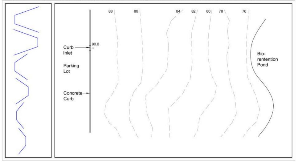
Place the appropriate contours on the site plan to maximize the amount of fill. Place the contours.
