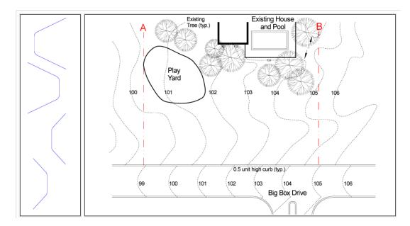
8. Refer to the exhibit(s). Grade the proposed parking garage entry ramp. Parking garage deck elevation must be a minimum of 4 units above bedrock. Place the appropriate spot elevation in the boxes provided.
