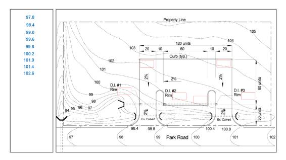
7. Refer to the exhibit(s). Place the appropriate contour(s) on the site plan to create a 0.5 unit high berm along the existing street between A and B.
