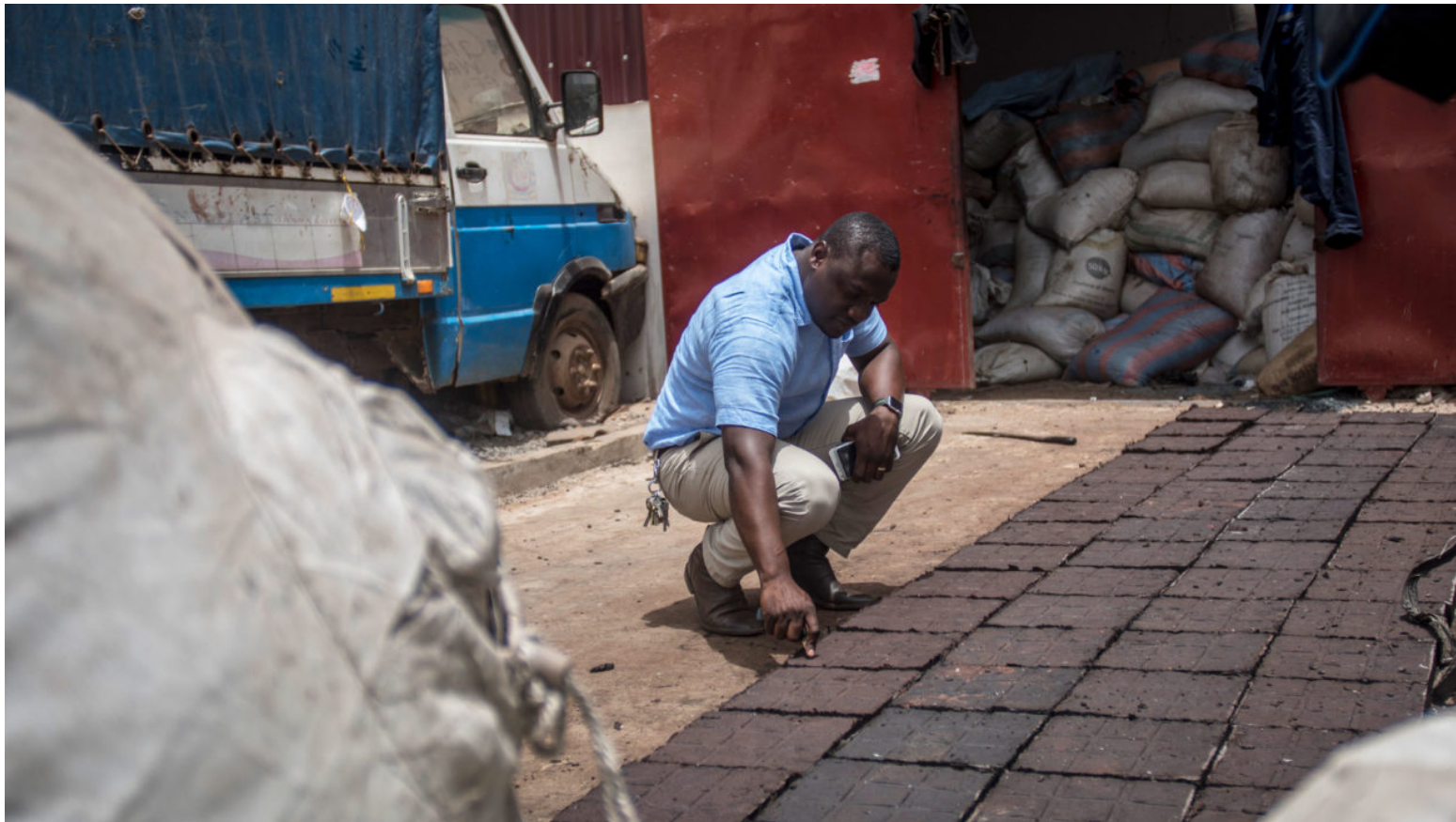
An engineer inspects paving blocks made from recycled plastics in a suburb of Accra, Ghana. CRISTINA ALDEHUELA/AFP VIA GETTY IMAGES
