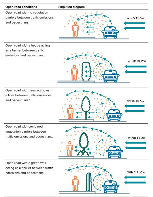
\*Under some conditions, due to a windbreak effect, pollutants can stagnate behind a sparse row of trees, leading to deteriorated downwind air quality (Abhijith and Kumar, 2019).
