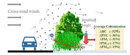
The above figure was extracted from Abhijith and Kumar (20191), who found pollutant concentration reductions downwind of hedge-tree combination barriers for BC (black carbon), PNC (particle number concentrations), PM1 (particulate matter with aerodynamic diameter <1  $\mu$ m), PM2-5 (particulate matter with aerodynamic diameter <2.5  $\mu$ m), and PM10 (particulate matter with aerodynamic diameter <10  $\mu$ m).
