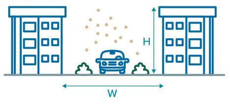
*H* is the height of the buildings and *W* is the horizontal distance between the buildings. The ratio of *H* to *W* is called the aspect ratio, which significantly affects pollutant dispersion patterns. For simplicity, street canyons can be broadly defined according to their aspect ratio.
