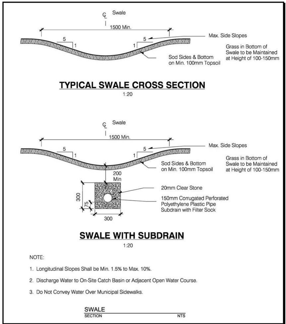
Figure 2-10: Typical swale cross section
