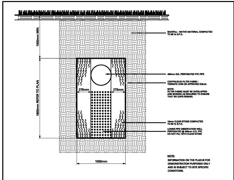
Figure 2-8: Cooling trench – profile section
