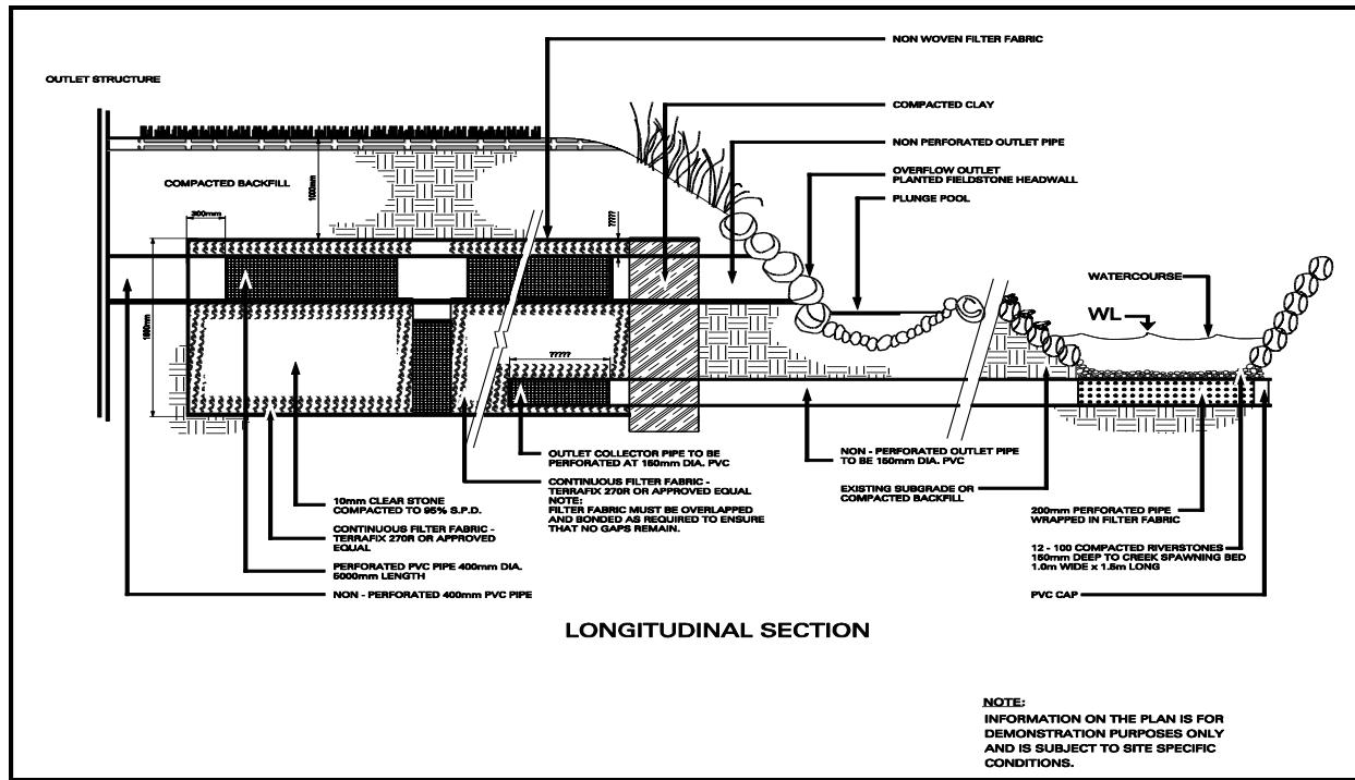
Figure 2-7: Cooling trench – longitudinal section
