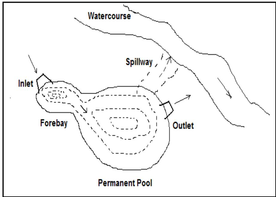
**Figure 2-3: A typical stormwater management pond**
