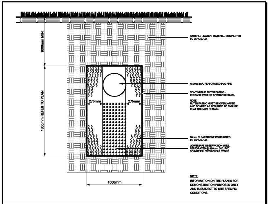
Figure 2-8: Cooling trench – profile section
