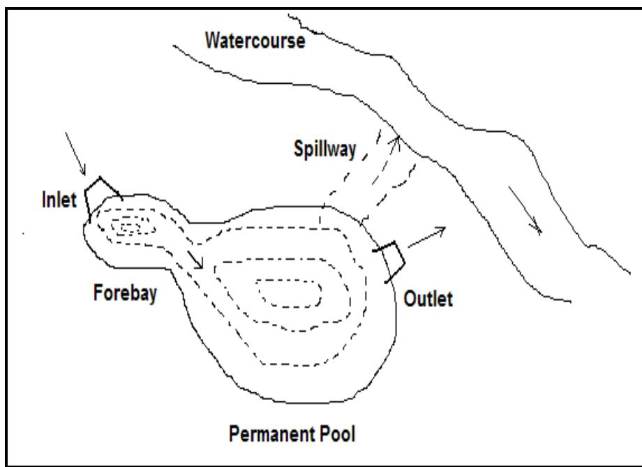
**Figure 2-3: A typical stormwater management pond**
