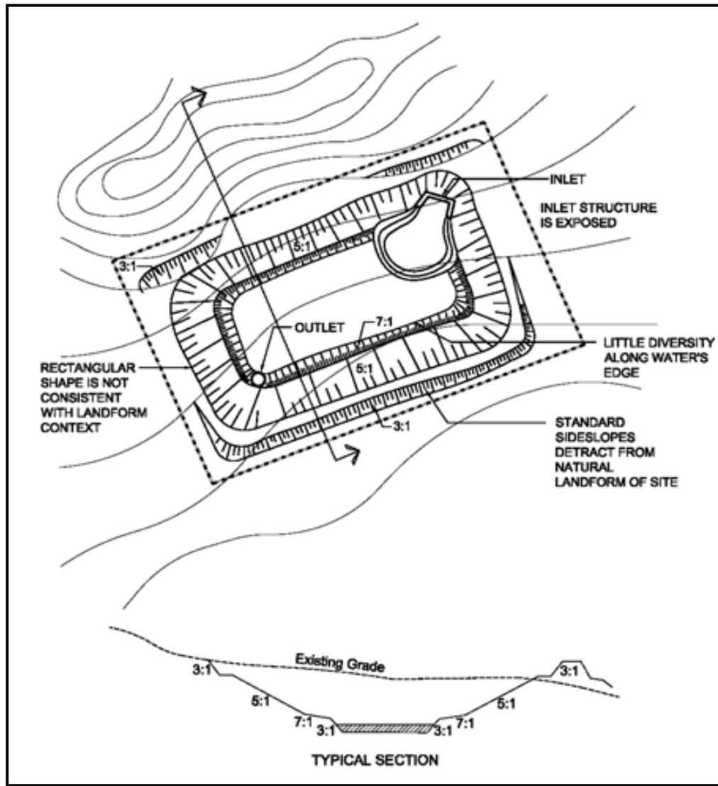
Figure 2-2: Planar Grading Design – Not Recommended <sup>1</sup>
