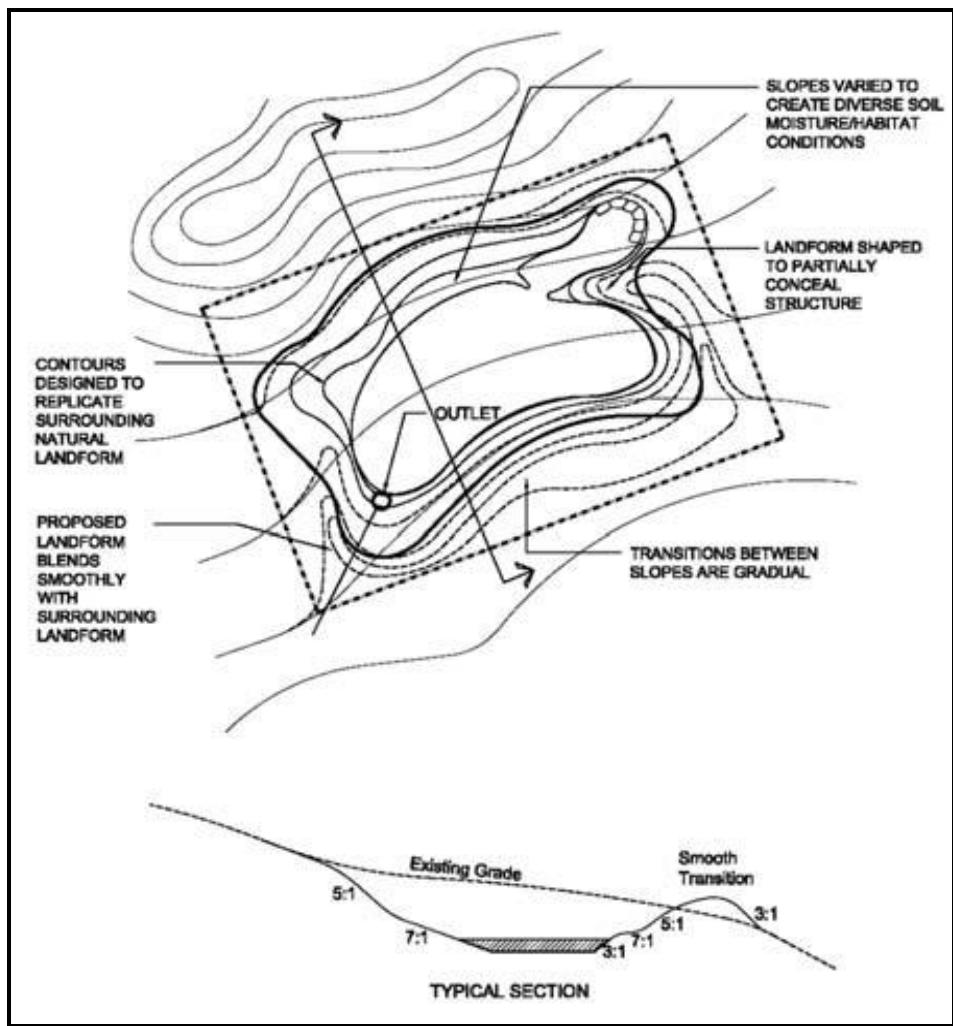
Figure 2-1: Landform Grading – Recommended Design <sup>1</sup>
