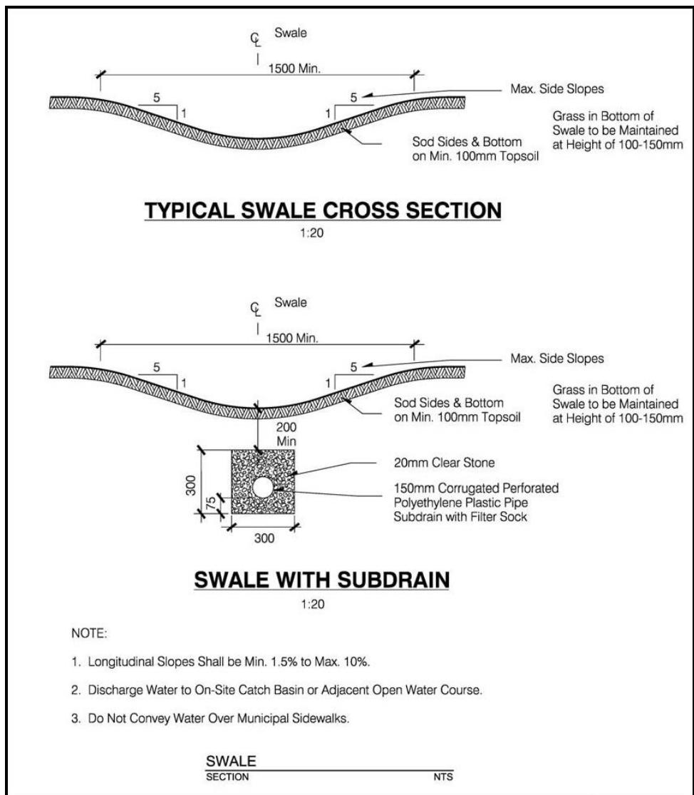
Figure 2-10: Typical swale cross section
