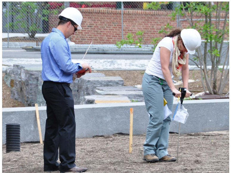
Figure 7. Soil Penetrometer Field Demonstration (Credit: Andropogon Associates)
