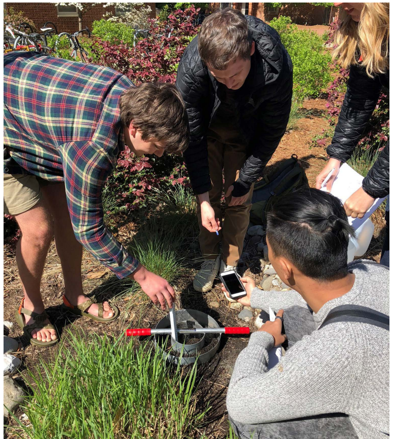
Figure 8. Double-ring Infiltrimeter Field Demonstration (Credit: Emily McCoy)
