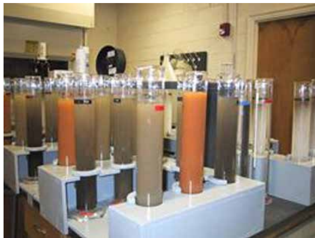
Figure 9. Particle size analysis sedimentation cylinders for determining percent of sand, silt, and clay of soil sample
