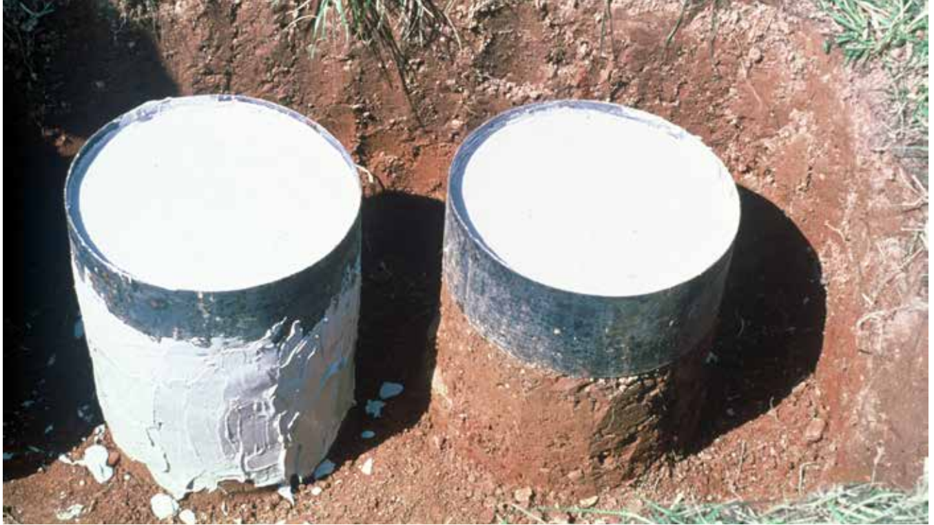
Figure 4. Soil pedestals for in-situ saturated and unsaturated hydraulic conductivity testing, Charlotte, NC
