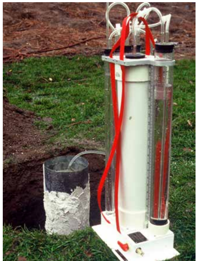
Figure 25. Constant head permeameter, New York, NY
