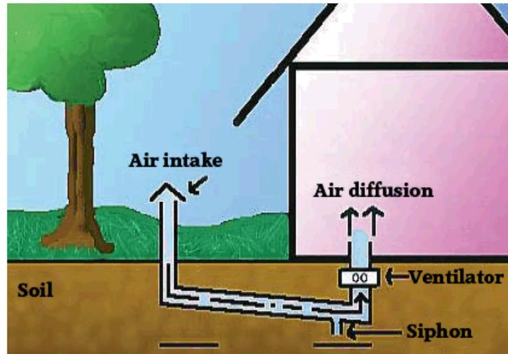
**Figure 9** Cross-section of a ground-coupled heat exchanger
