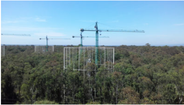
Rings of white tubes pump elevated levels of CO 2 onto eucalyptus trees at a research site near Sydney, Australia. Courtesy of Belinda Medlyn
